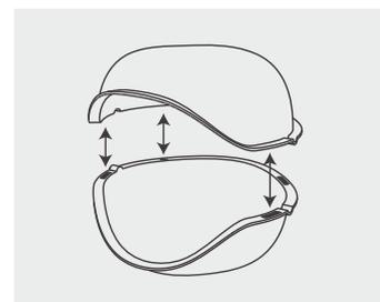
Join the shells vertically using the supplied face fastener and the two shells are firmly fixated.
